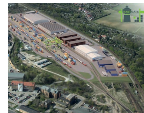
This is how it will look like in the future at the CT terminal in Frankfurt (Oder): Beside the construction of additional tracks and the installation of a cross-tracks crane runway, new areas for the settlement of rail-specific logistic companies are being developed.
